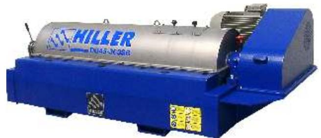
While the solids particles settle to the bowl wall and are discharged by means of a screw conveyor, the cleared liquid phase accumulates above the sedimented solids phase and is discharged at the opposite end of the machine.
